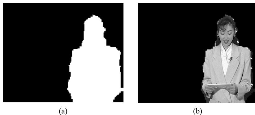
Figure 8. (a) The final object mask. (b) The result of the object extraction.
